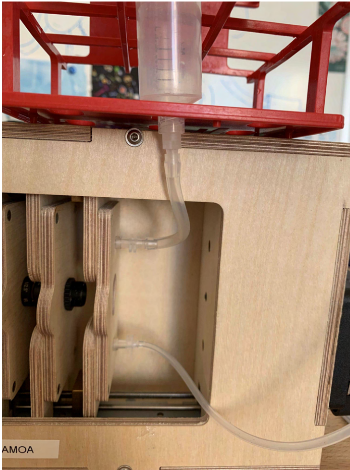
example of optimised setup to avoid long path between sample and flowcell
