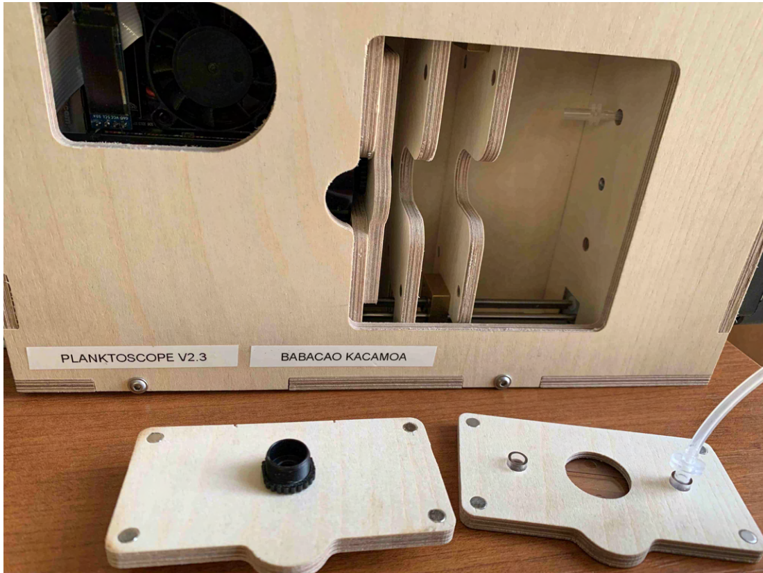
objective lens and flowcell removed
