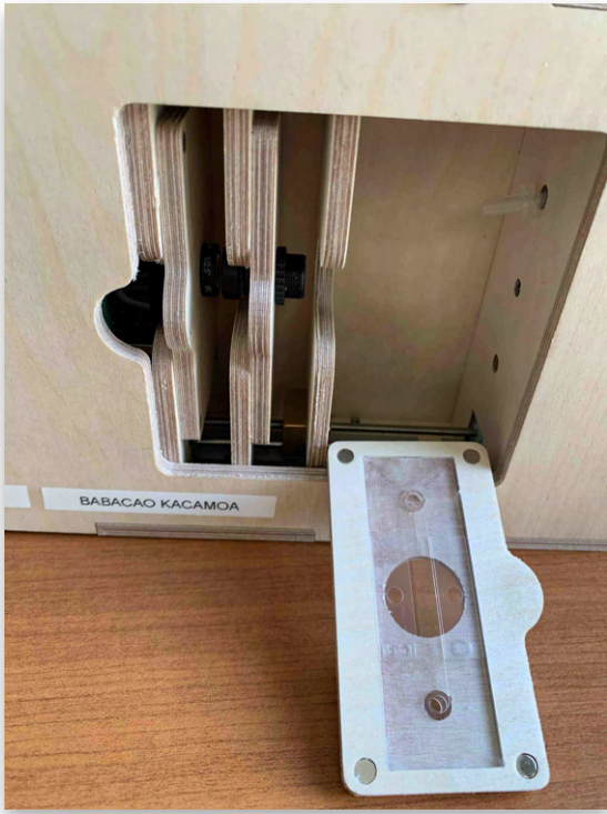
tube / objective lenses in place. Ibidi flowcell on its stage
