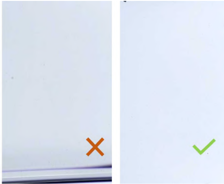
Figure 4: The figure on the left shows a misaligned Flow Cell. The background should be homogeneous like in the figure on the right.
