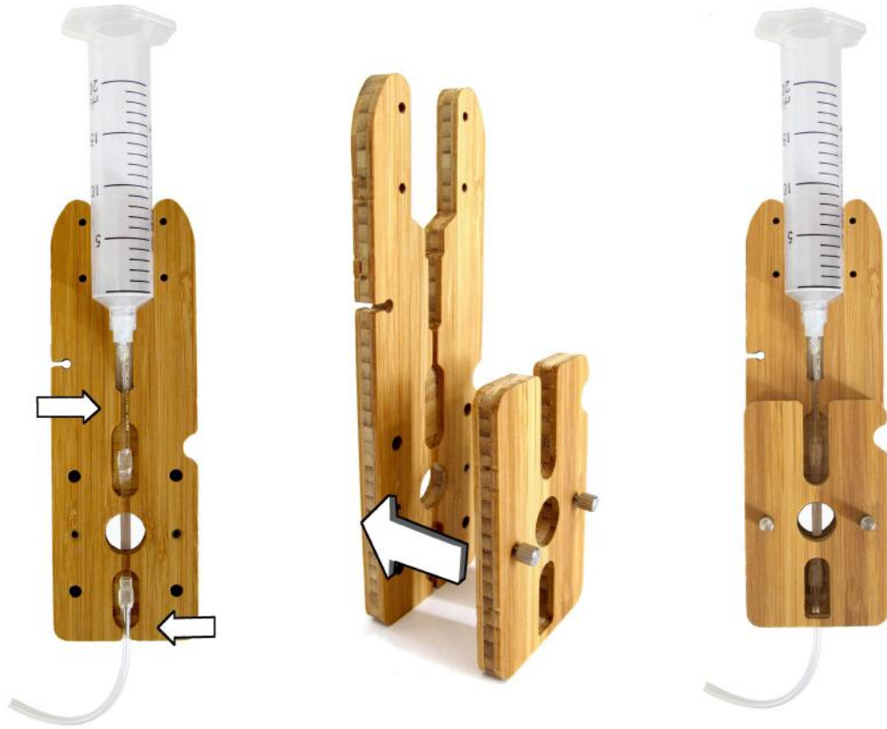
Figure 5: How to install the Flow Cell. You will need the syringe (F6), the Flow Cell holder (E) and one Flow Cell (H).
