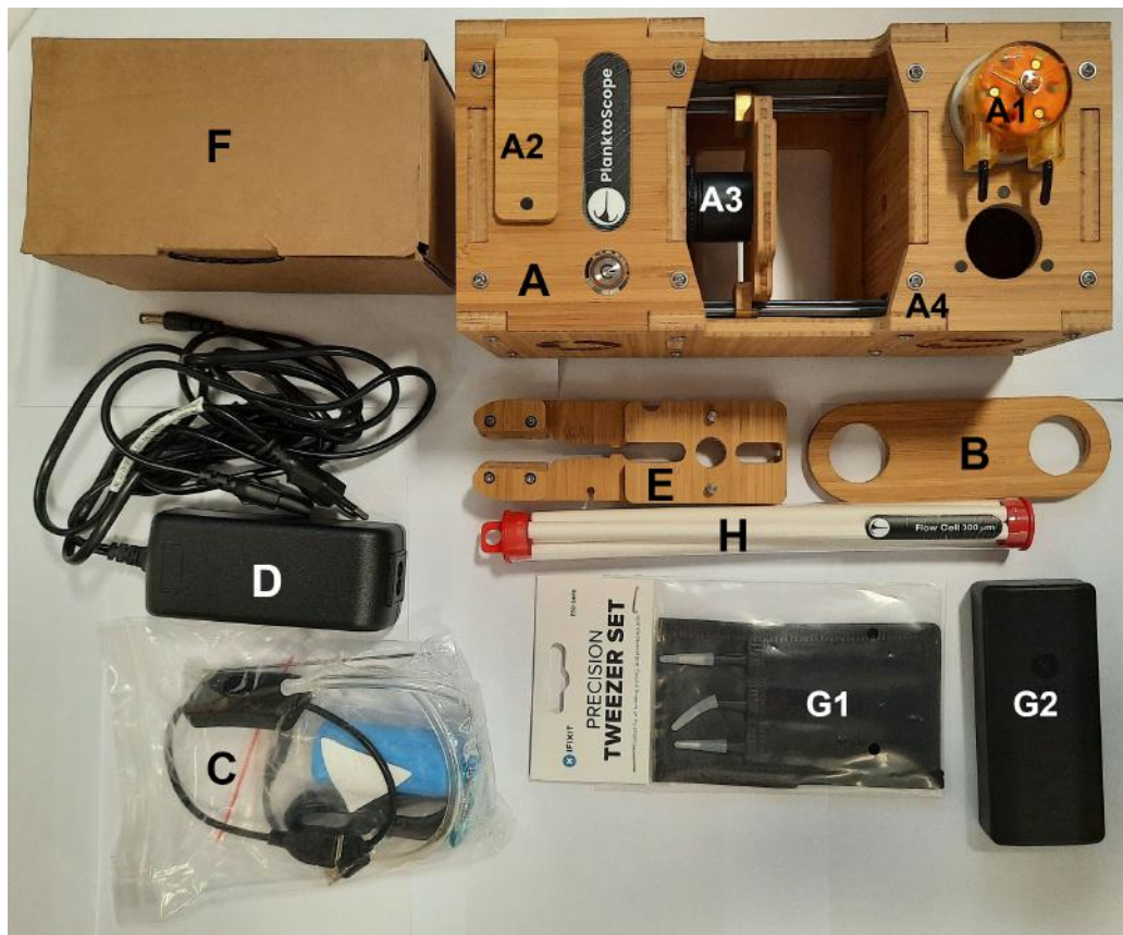
Figure 1: The PlanktoScope Kit. (A) The main box with the pump A1, the USB cover A2, the pi camera A3 and the screws A4; (B) Tube holder; (C) Bubbler; (D) Power cable; (E) Flow Cell holder; (F) Supplementary materials box; (G) IFixit kit; (H) Flow Cell
